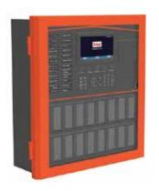
The TX7008 is designed to provide early warning fire detection, to quickly identify the location of fire and provide user definable text informing the occupants of the building of potential smoke spread. Simultaneously, the TX7008 will alert and evacuate the occupants, and control all necessary auxiliary command functions such as elevator control, air handling shut down, gas shut off & damper control, as per the cause and effects requirements configured though Command Builder Set-up.
